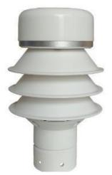
between the speed rate and the size of drops, the quantity of rain or its intensity will be registered. The rain/precipitation type (rain/snow/snow-covered rain/freezing rain/hail) is determined thanks to the speed rate of the rain. Resolution up to 0.1mm, without maintenance.
